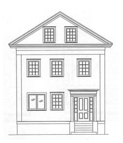
**1 Inappropriate** Replacement single-pane casement window with enlarged opening. Missing drip caps.
