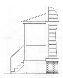
**1 Inappropriate** Metal pipe railing. Lack of detailing on column and railing. No visual support for column. No stair nosing.
