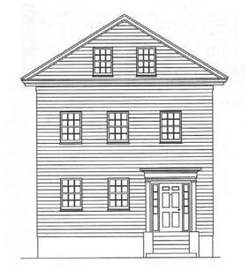
**Inappropriate** Aluminum or vinyl siding. Loss of cornerboards, window trim and other details.
