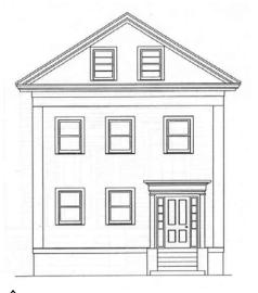
**1 Inappropriate** Horizontally divided window replacements have incorrect number of panes. Missing drip caps.
