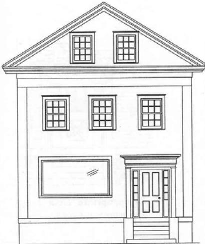
↑ **Inappropriate** Enlarged window opening for picture window.
