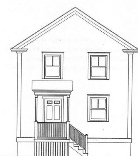
↑ **Inappropriate** Support for columns has been covered over.
